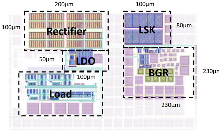
Fig. 8. System Layout diagram. The individual core electronic blocks are detailed, along with their dimensions.
