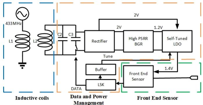
Fig. 1. The system consists of three blocks: Inductive coil, data and power management, and front end sensor. The secondary coil  $L_2$  receives wireless power from the external circuit and feeds this AC power to a rectifier. A high PSRR BGR after the rectifier is responsible for providing a stable voltage for the self-tuned LDO circuit, which is capable of down-converting the 2V supply to a regulated 1.4V voltage supply for front end sensor.
