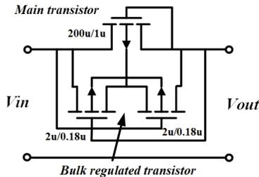
Fig. 3. Bulk regulated circuit. It should be connected to all the transistors in the rectifier.
