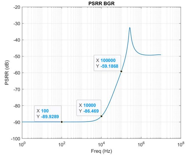
Fig. 9. Simulated PSRR of the BGR in this work. It achieves a PSRR of -59dB at 100kHz with a power consumption of 61 µW.
