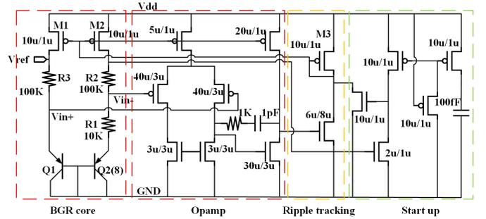
Fig. 4. The High-PSRR BGR schematic consisting of four parts - the core, opamp, ripple tracking and start up circuits.
