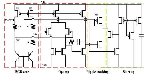
Figure 4 High-PSRR BGR schematic
