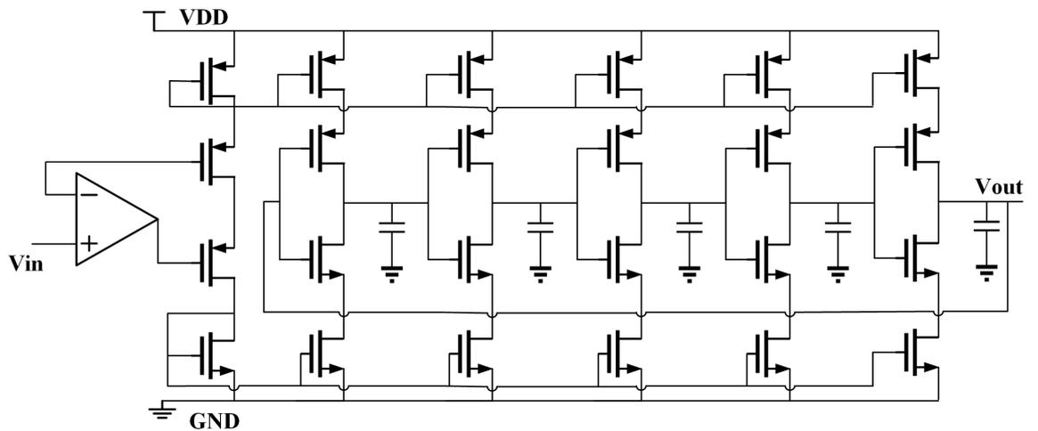
Figure 5.4: Schematic diagram of the voltage controlled oscillator.
