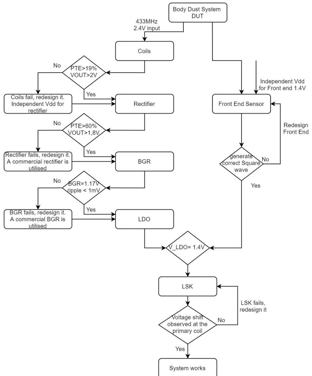
Figure 6.4: The Body Dust system test plan flow chart.
