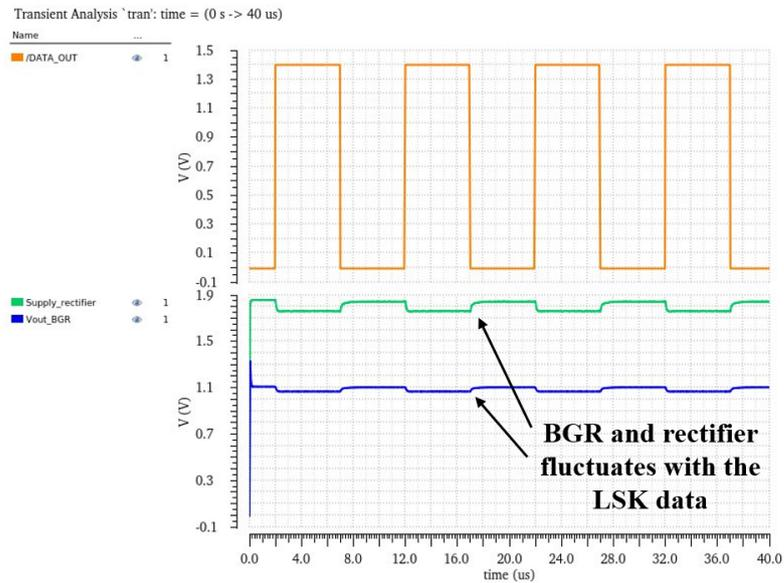
Figure 4.12: Voltage reference (blue line) is affected by the high frequency power supply.
