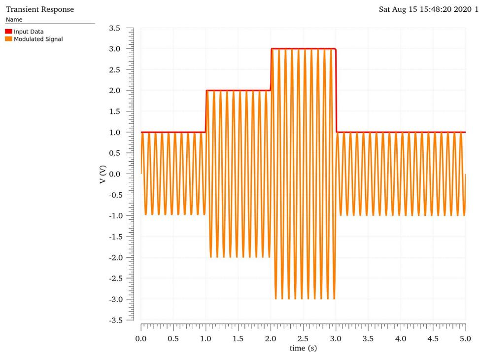
Figure 5.7: An example of ASK modulation. The carrier amplitude changes according to a digital input signal. The modulation technique buries the digitised data in the envelop of the carrier signal.
