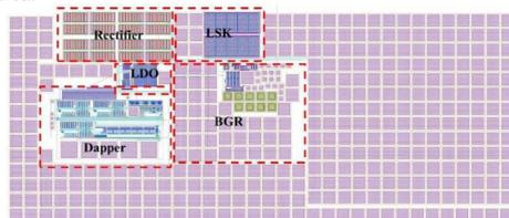
Figure 9 System Layout diagram
