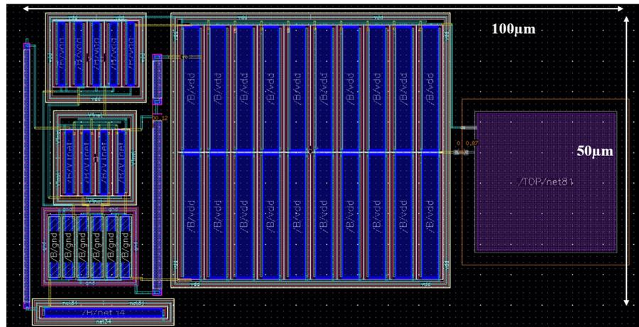
Figure 4.26: The layout diagram of self-tuned LDO.
