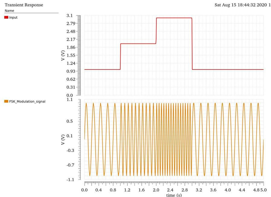
Figure 5.8: An example of FSK modulation. The carrier frequency changes according to a digital input signal.
