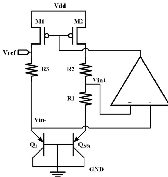
Figure 4.11: Schematic of a basic BGR.
