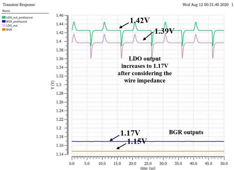
Figure 4.27: The post layout co-simulation of LDO with BGR with respect to time.
