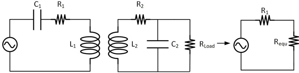
Figure 3.3: The simplification of the inductive coil circuit.
