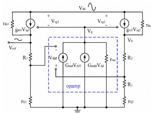
Figure 4.13: The small signal analysis model of conventional BGR [4].
