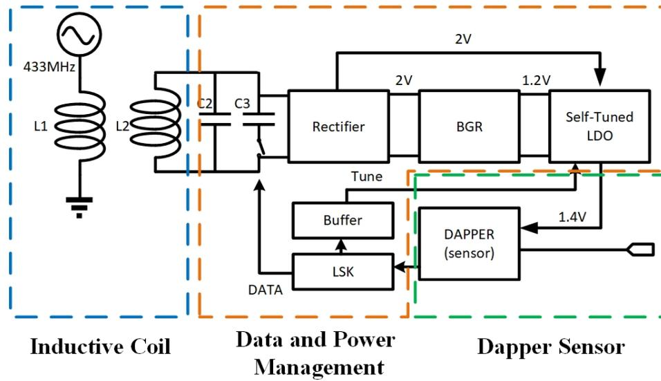
Figure 3.1: Body dust system architecture.
