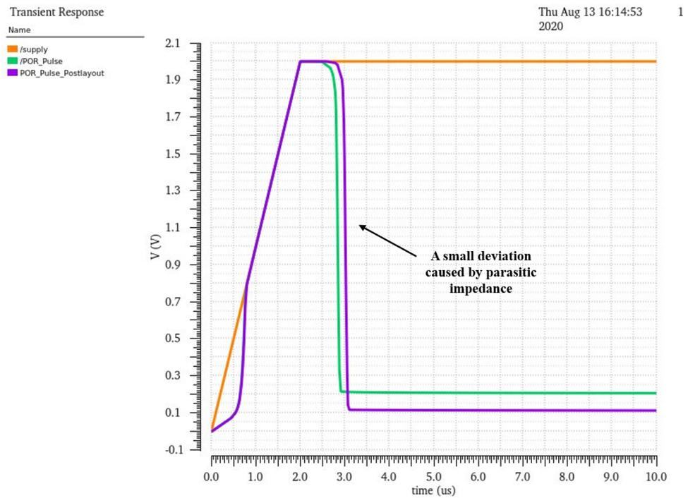
Figure 4.33: Post-Layout simulation of the POR circuit.
