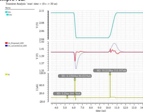
Figure 7 simulated response of the conventional and the self-tuned LDO circuit.
