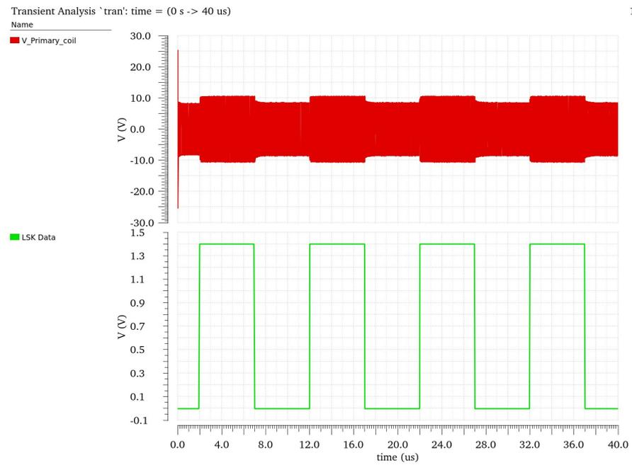
Figure 5.12: The simulation waveform of LSK circuit. Once an LSK data triggers the LSK switch, a voltage shift across the primary side can be observed.
