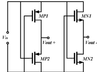
Figure 2 Fully cross-coupled rectifier
