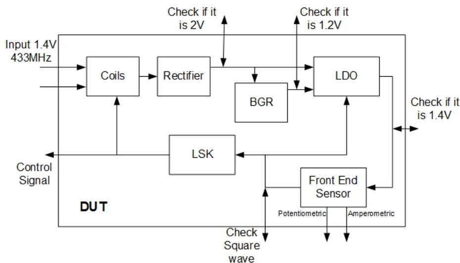
Figure 6.3: The Body Dust system test plan diagram.
