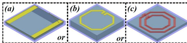
Figure 4.1: Diagram of three different coil designed by Dr. Peilong [1]. (a). around CMOS, (b) above-CMOS, (c) in-CMOS
