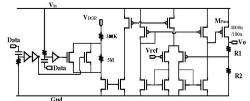
Figure 6 the proposed self-tuned LDO circuit
