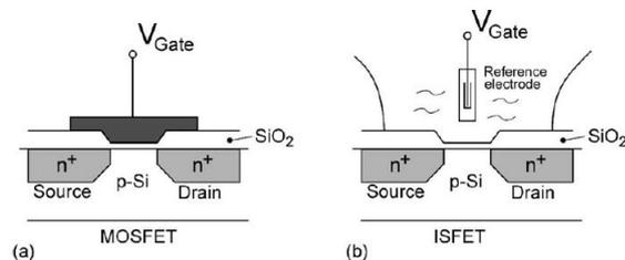
Figure 5.1: Schematic of MOSFET and ISFET [5].
