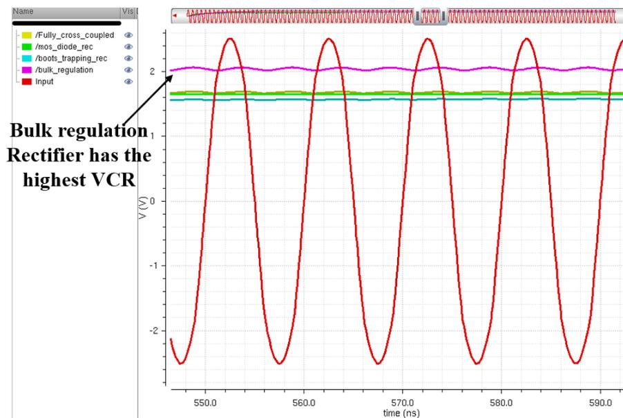
Figure 4.6: Waveforms of different topology of rectifiers.
