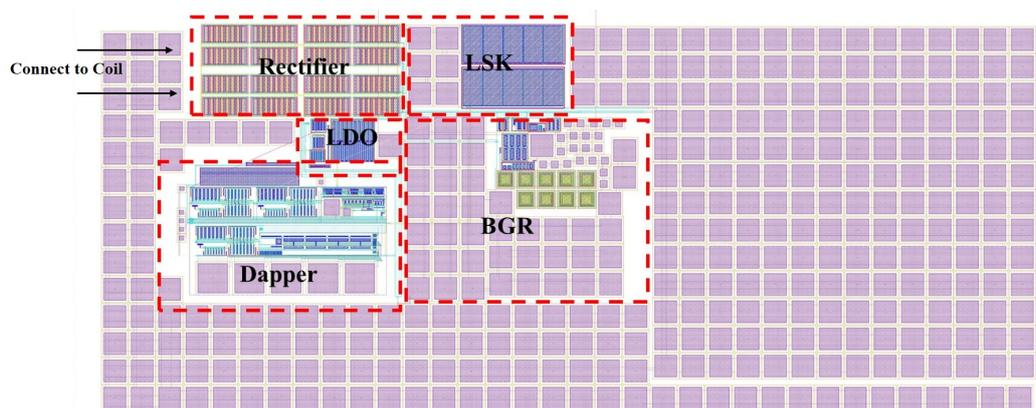
Figure 6.2: The Body Dust system layout. A large area smoothing capacitor is surrounding around the circuit.
