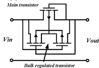
Figure 3 Bulk regulated circuit
