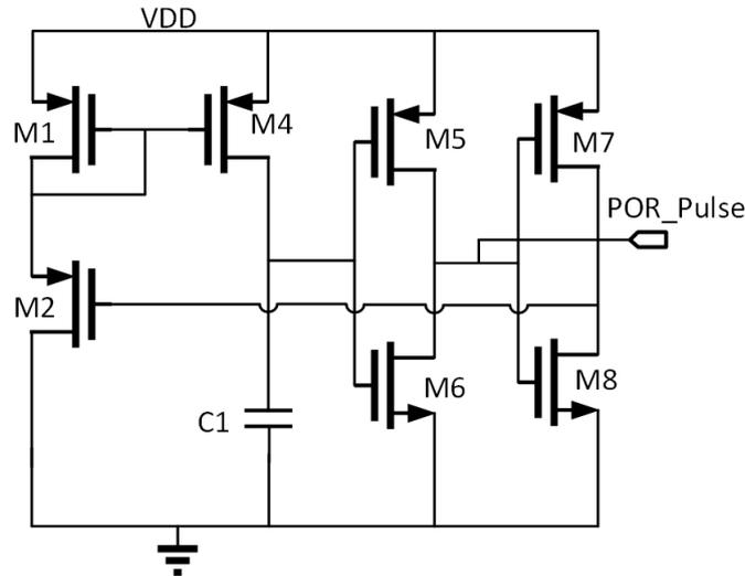
Figure 4.30: Schematic diagram of the proposed POR circuit
