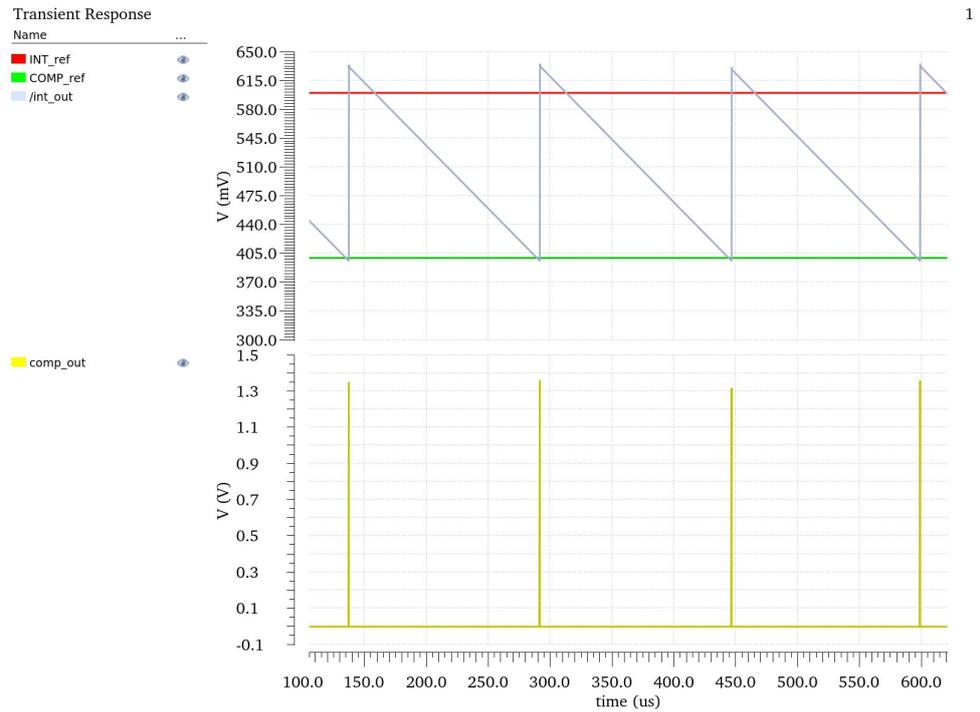
Figure 5.3: Waveform of the amperometric circuit. The comparator output triggers once the integrator output reduces below  $COMP\_ref$ .
