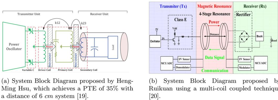
Figure 2.1: Two block diagram of the state-of-the-art WPDT system
