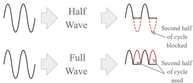
Figure 4.3: The wave output from halfwave rectifier and fullwave rectifier [3].
