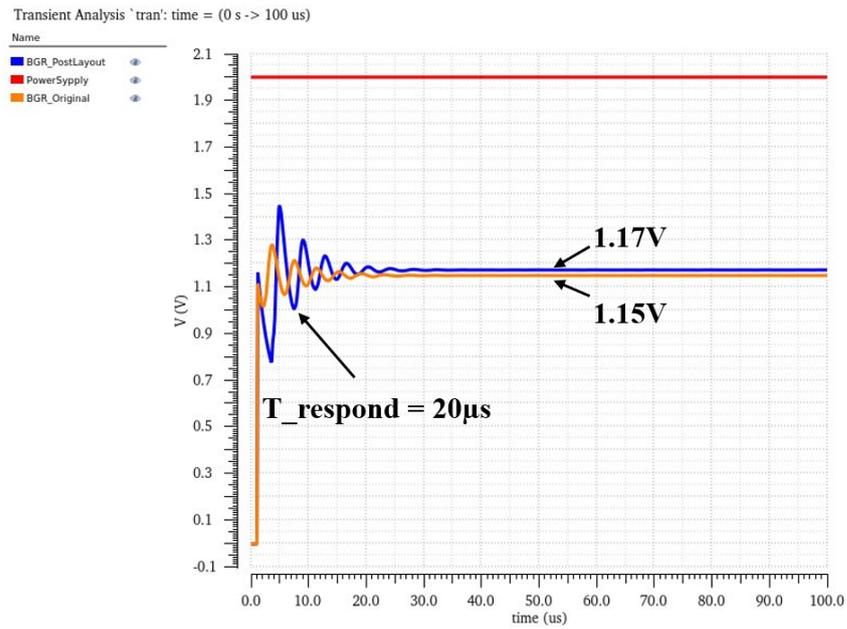
Figure 4.19: The comparison between the original BGR output and the post-layout BGR Output.
