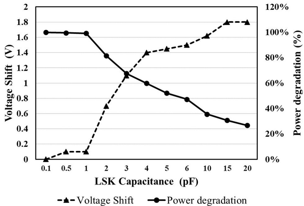
Figure 5.11: The line diagram of Voltage shift and PTE degradation with respect to different LSK Capacitance. When  $C_3$  and  $C_4$  in Figure 5.10 equal to  $3pF$ , they achieve the best balance between voltage shift and PTE
