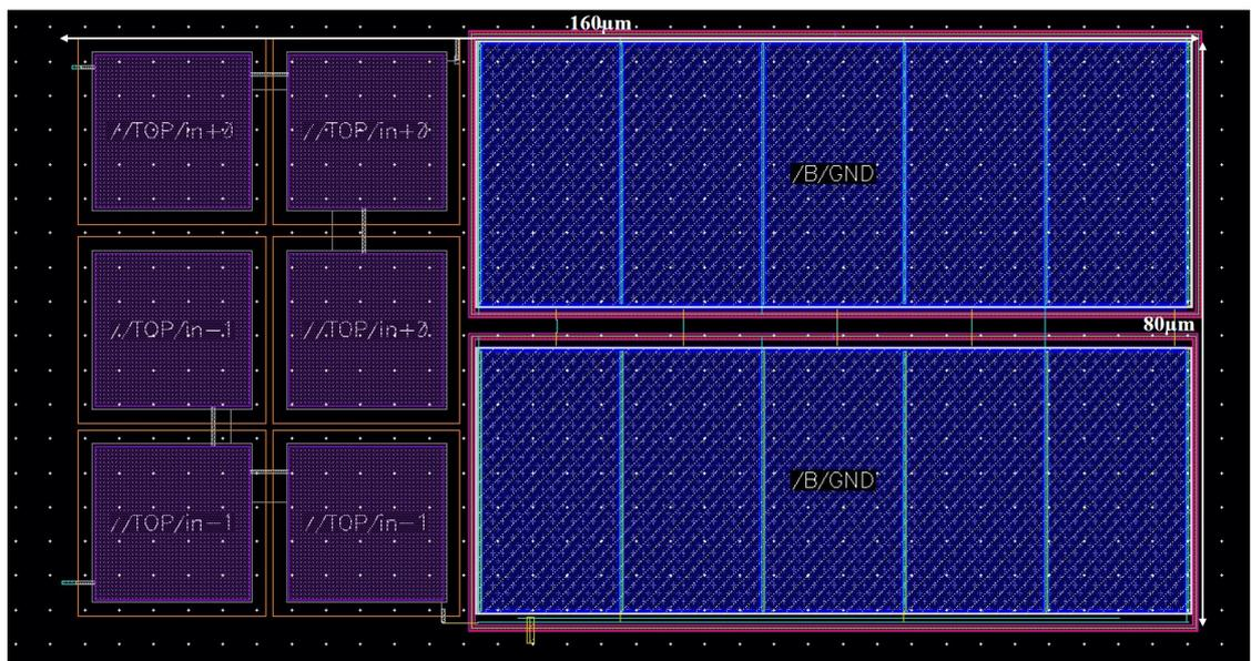
Figure 5.13: The layout diagram of the LSK circuit.
