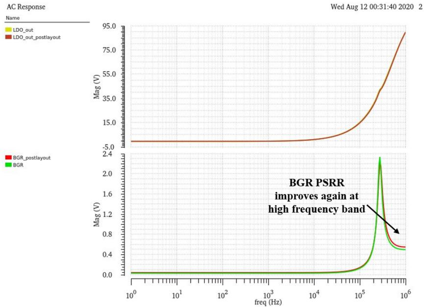
Figure 4.28: AC response of the LDO and BGR co-simulation before and after post-layout extraction.
