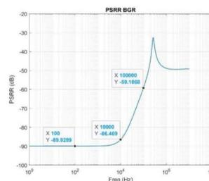
Figure 11 simulated PSRR of the BGR in this work
