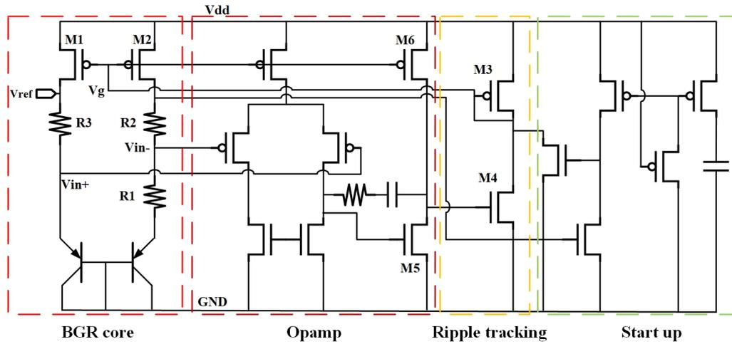
Figure 4.14: Schematic diagram of a high PSRR BGR .
