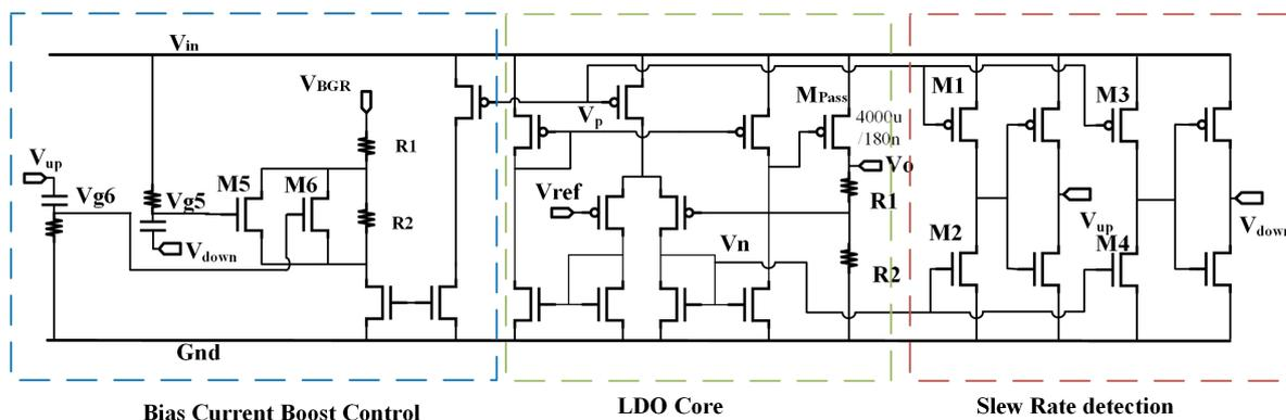
Figure 4.22: Schematic diagram of a dynamic bias current LDO. It consists of three blocks: a bias current boost control block, a LDO core and a slew rate detection
