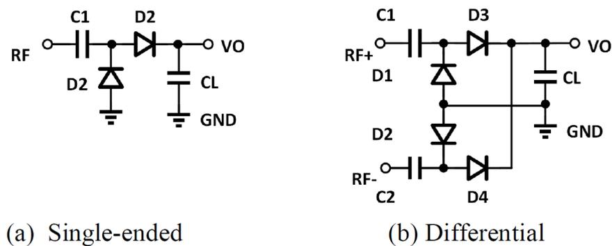
Figure 4.2: Schematics of single ended and differential rectifier [3].
