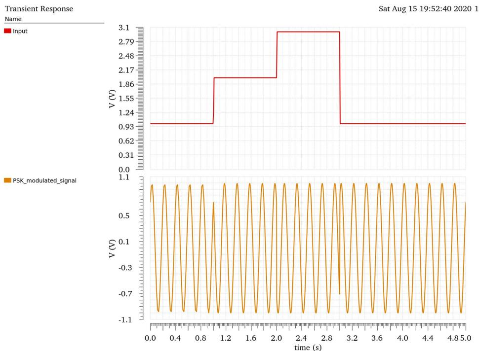
Figure 5.9: An example of PSK modulation. The carrier signal phase is varied with a digital input signal.
