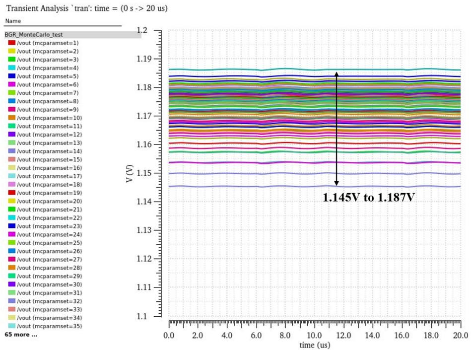
Figure 4.20: A MonteCarlo test of 100 runs of BGR.
