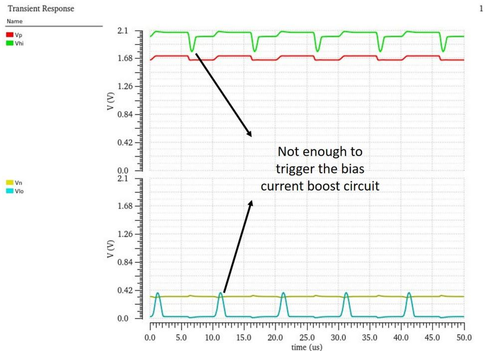
Figure 4.23: Waveform of a dynamic bias current LDO, the internal detection node is not strong enough to trigger the bias current boost circuit
