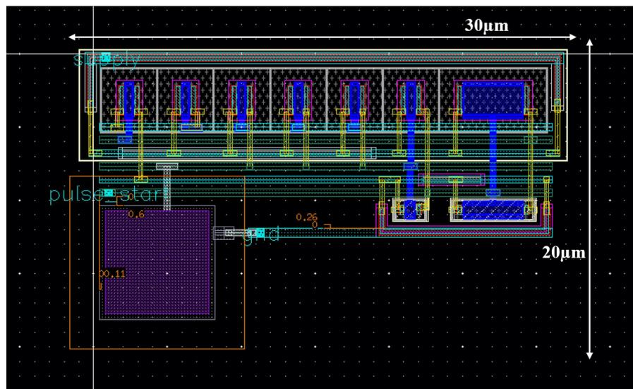
Figure 4.32: Layout diagram of the POR circuit.
