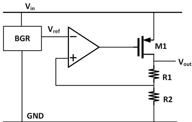
Figure 4.21: Schematic diagram of a conventional LDO.
