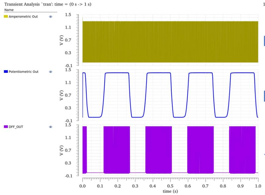
Figure 5.6: Simulation waveform of the Dapper Sensor. The output signal mixes the amperometric signal and the potentiometric signal
