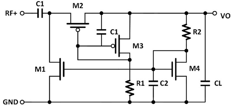
Figure 4.4: Schematic of a  $V_{th}$  cancellation rectifier.
