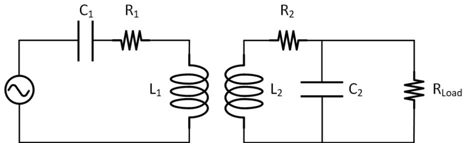
Figure 3.2: A conventional Inductive coil circuit.
