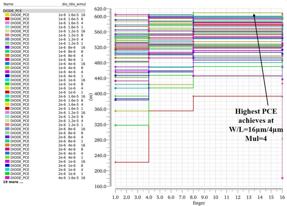
Figure 4.8: Different size of diodes are compared to achieve the highest PCE. The best fit is found at the  $W/L = 16\mu m/4\mu m$  and multiplier=4.
