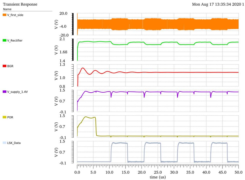
Figure 6.1: The Body Dust system level simulation diagram.
