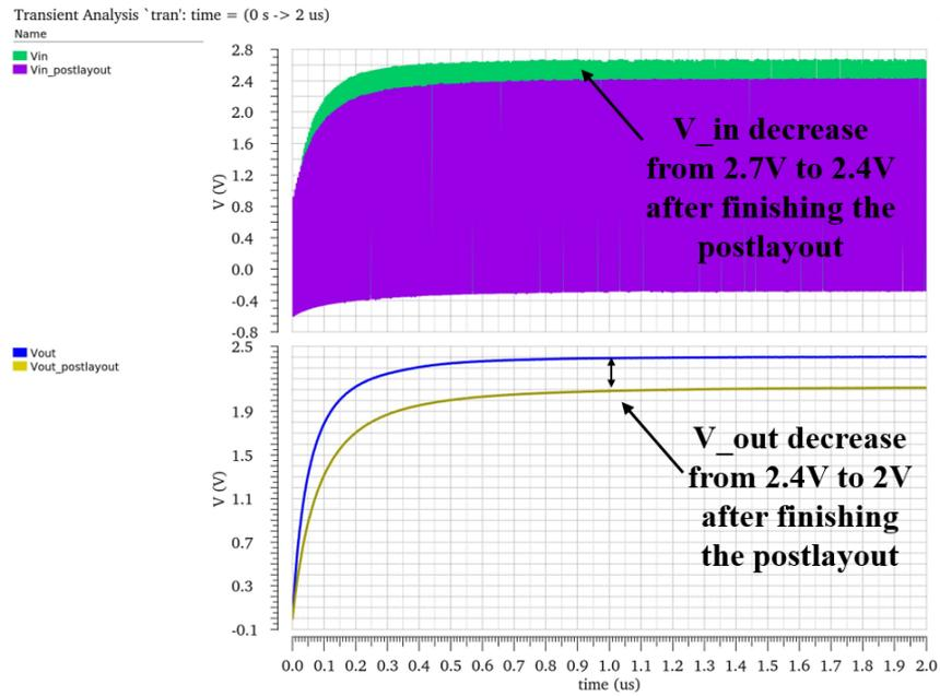
Figure 4.10: The simulation waveform of post-layout rectifier.
