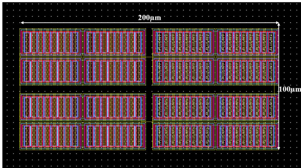
Figure 4.9: Shottky diode rectifier layout.
