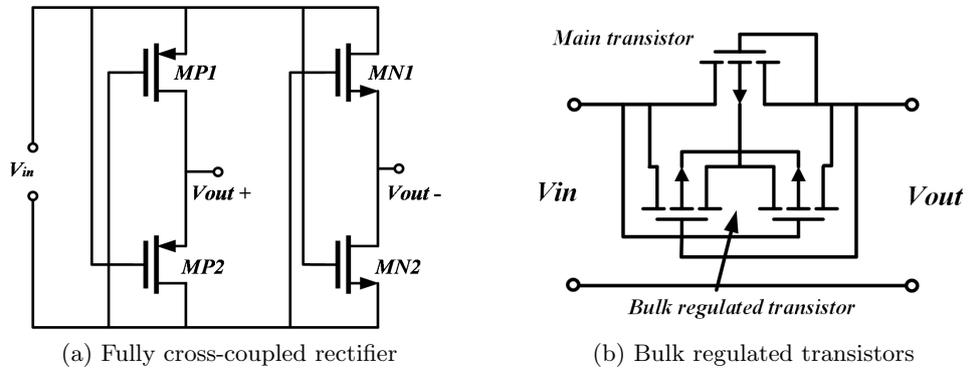
Figure 4.5: The bulk regulated transistors are added to every transistors in fully cross-coupled rectifier, ensuring the main transistor's source terminal are always connected to the lowest potential
