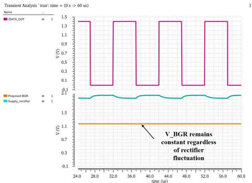
Figure 4.15: Waveform of the proposed high PSRR BGR .
