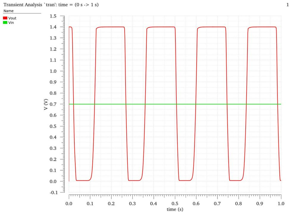
Figure 5.5: Simulation waveform of the voltage controlled oscillator. Voltage input is converted to a square wave with a certain frequency.
