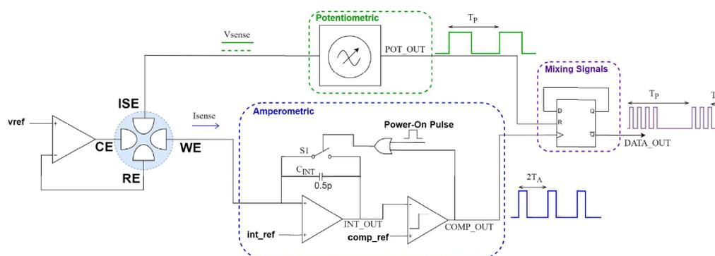
Figure 3.5: Front end sensor system architecture [2].
