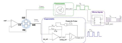
Figure 8 Dual amperometric and potentiometric sensor [5]
