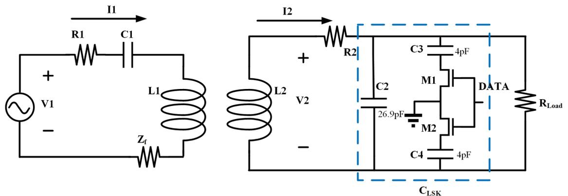
Figure 5.10: The Schematic diagram of LSK circuit.
