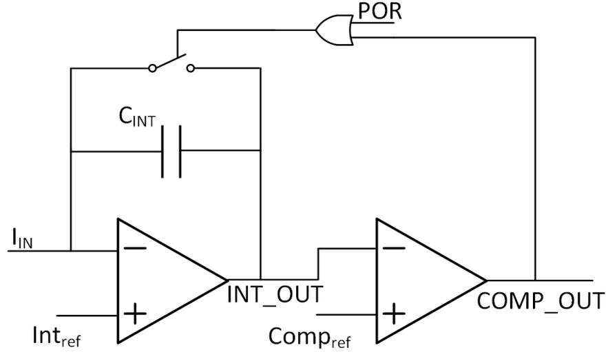
Figure 5.2: Schematic of amperometric readout circuit.
