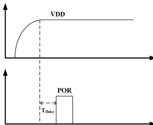
Figure 4.29: A POR pulse will trigger by a threshold level detection.
