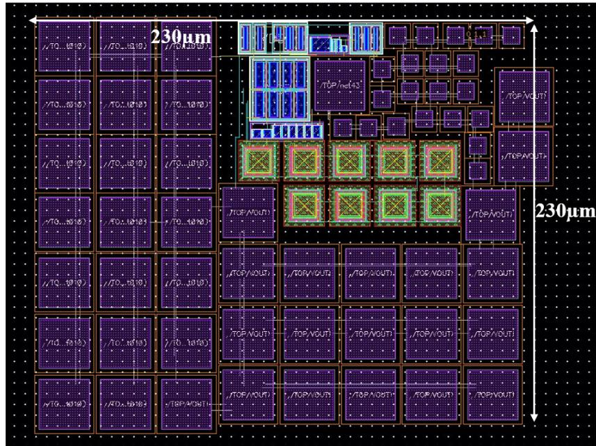
Figure 4.18: The diagram of layout the proposed BGR and a large area of capacitor is used to smooth the voltage reference.
