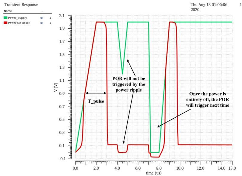
Figure 4.31: Waveform of the POR circuit. the red line shows the POR signal and green line show the power supply.
