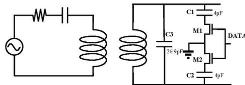
Figure 5 A wireless power and data transmission system with a LSK circuit
