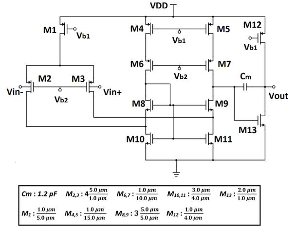
Fig. 4. Folded cascode op-amp A1 with transistor dimensions, adapted from [5, Fig. 4a].
