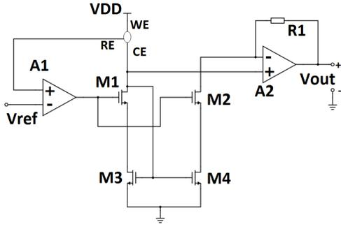
Fig. 2. Reference potentiostat topology, adapted from [5, Fig. 2].
