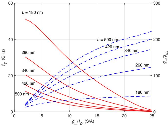
Fig. 1.  $f_T$  and  $g_m/g_{ds}$  against  $g_m/I_D$  for a range of lengths;  $V_{DS} = 0.9$  V;  $V_{SB} = 0$  V; N-channel IGS in TSMC 180 nm.
