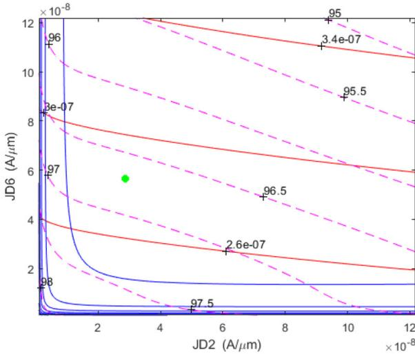
Fig. 5. Optimised design contour curves for two-stage op-amp A2. Total DC current (nW, red), total active area ( $\mu\text{m}^2$ , blue), and total gain (dB, dashed magenta) contour curves. The selected point is marked by the green dot.
