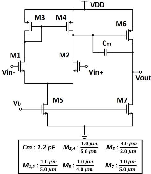
Fig. 3. Two-stage op-amp A2 with transistor dimensions, adapted from [5, Fig. 4b].
