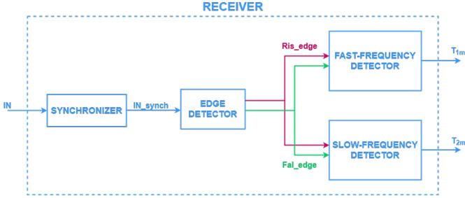
Fig. 4. Top level view of the receiver. This architecture consists of four building blocks: (1) a synchronizer, (2) an edge-detector, (3) a fast-frequency detector, and (4) a slow frequency detector.
