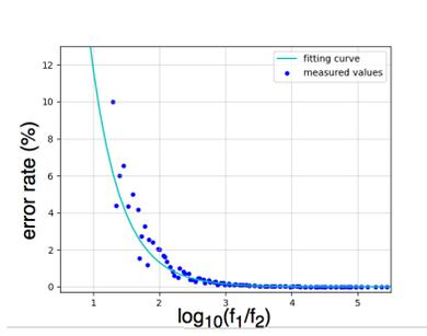
Fig. 7. Average error on  $T_2$ , showcasing the error from the results collected in the simulations averaged over different  $\Delta\phi$  for each  $\frac{f_1}{f_2}$ . The fitting curve shows the general trend.
