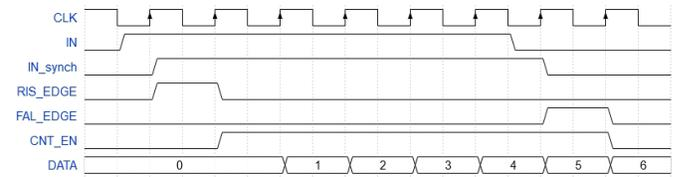
Fig. 6. Example of timing diagram related to the high-pulse counting process at the receiver. IN is the asynchronous input signal. IN\_sync represents the synchronous version of the receiver input signal, whose pulse length is the same as the one of the CNT\_EN signal, which demonstrates that no further error arise during the edge detection.
