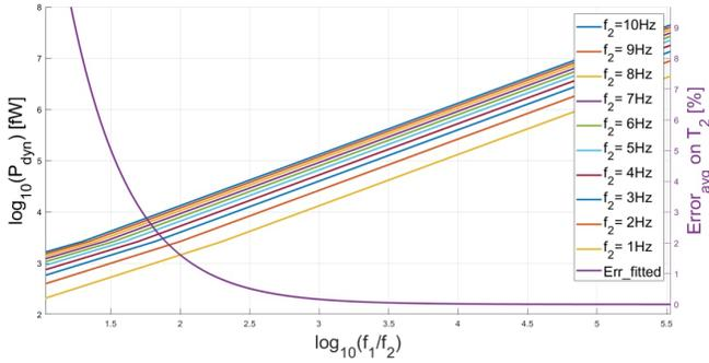
Fig. 12. Combined (1) error and (2) power plots. (1) is the fitting curve of the average error on  $T_2$  red as shown in Fig. 7. (2) is a set of straight lines for different  $f_2$  representing the dynamic power consumed in the mixer as a function of  $\frac{f_1}{f_2}$ .
