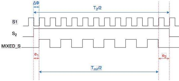
Fig. 11. Example of timing diagram of digital mixing. The error on  $T_2$  generated in the mixed signal is equal to the 12%. The relative phase shift among  $S_1$  and  $S_2$  is of the 50%, and the frequency ratio is equal to 25.
