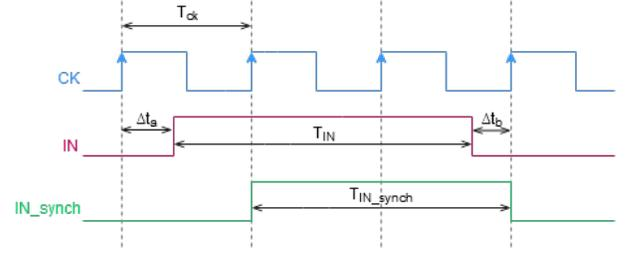
Fig. 5. Timing diagram related to the synchronization stage at the receiver side and the error on the resulting synchronized signal
