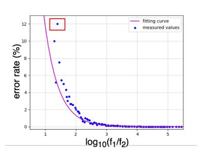
Fig. 8. Maximum error on  $T_2$ , showcasing the maximum error from the results collected in the simulations for specific  $\Delta\phi$  and  $\frac{f_1}{f_2}$ . The section in red shows that the error overcomes the limit of the 10%.
