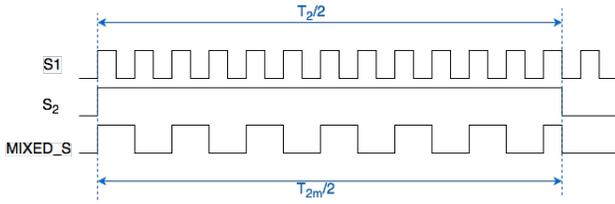
Fig. 10. Example of timing diagram of digital mixing.  $T_2$  is the period of the input signal  $S_2$ , while  $T_{2m}$  is the period of  $S_2$  in the mixed signal. No error on  $T_2$  is generated in the mixed signal. The relative phase shift among  $S_1$  and  $S_2$  is of the 0%, and the frequency ratio is equal to 25.
