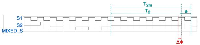
Fig. 2. Timing diagram of the signals involved in the mixing process and related errors on the output signal.  $\Delta\phi$  is the relative phase shift of the input signals ( $S_1$  and  $S_2$ ).  $T_2$  is the period of the signal with the lower frequency (i.e.  $S_2$ ).  $T_{2m}$  is the period of  $S_2$  in the mixed signal, that is characterized by a certain error  $e$  with respect to the original period  $T_2$ , and that arises from the input frequency ratio and from  $\Delta\phi$ .
