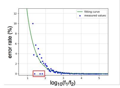
Fig. 9. Minimum error on  $T_2$ , showcasing the maximum error from the results collected in the simulations for specific  $\Delta\phi$  and  $\frac{f_1}{f_2}$ . The section in red shows that the error due to may reach the 0% even for sufficiently small frequency ratios.
