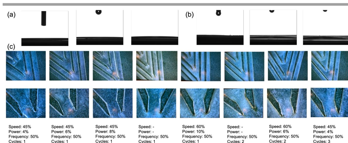
**Figure 3.** Investigation on hydrophilic tapes. (a) The DI water contact angles of the hydrophilic tape. (b) The artificial sweat contact angles of the hydrophilic tape. (c) Photos of the hydrophilic tape after laser cutting under a microscope, the laser cutter was set at a different speed, power, frequency, and cycles each time to test the optimum settings for the hydrophilic tape.
