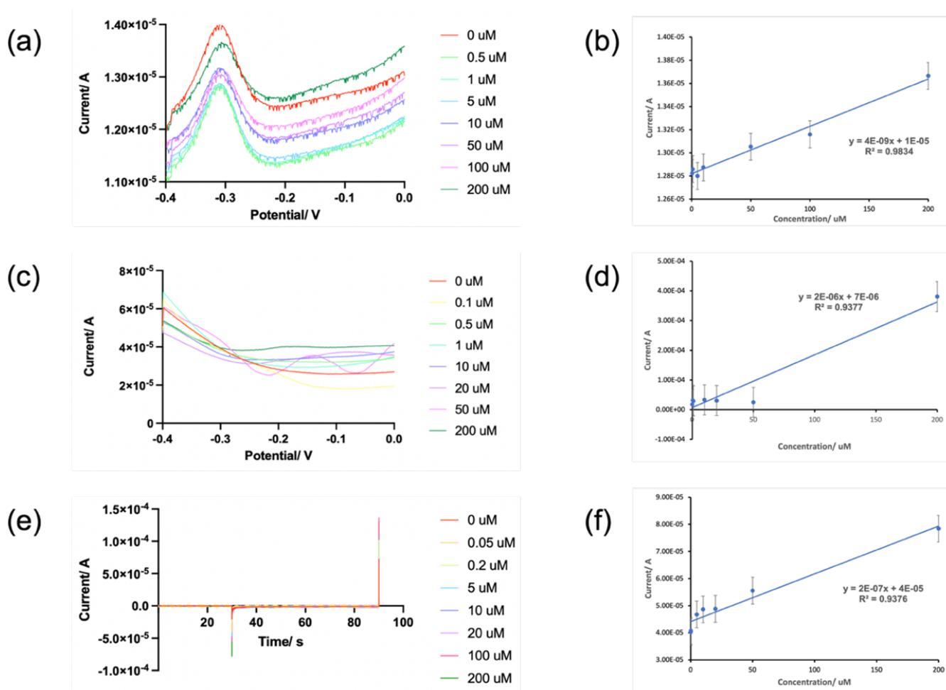
**Figure 4.** Voltammetry of different concentrations of penicillin G in (a) PBS solution and (c) artificial sweat at 10 mV/s from -0.4 V to 0 V with equilibration time of 15 s. (e) Chronoamperometry of penicillin G in artificial sweat. (b, d, f) Plots of electrochemical data.
