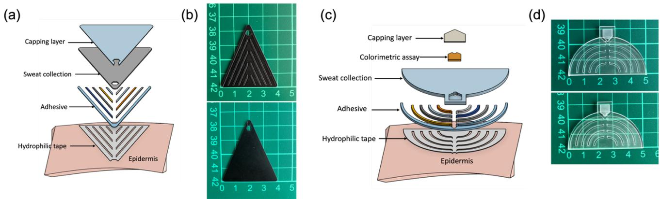
**Figure 6.** Schematic illustration and optical images of two epidermal microfluidic sweat devices. (a) Exploded view of the device highlighting various functional layers for electrochemical sensing. (b) Optical images of the device for electrochemical sensing. (c) Exploded view of the device highlighting various functional layers for colorimetric sensing. (d) Optical images of the device for colorimetric sensing.
