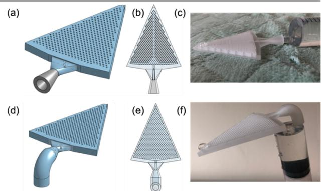
**Figure 7.** Images of the design and performance of the testing chips. (a, d) Shaded view and (b, e) transparent view of the chips to simulate the sweat generation process. (c, f) Optical images of liquid being injected into the chip.
